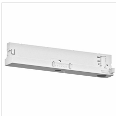
311063 Compact 4-conductor adapter with integrated driver (3-phase) (100-850 mA - max. 40 VDC)
